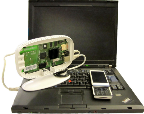
Figure 3. Our setup: A computer to monitor traffic and perform attacks, a victim phone and an SFR femtocell.
